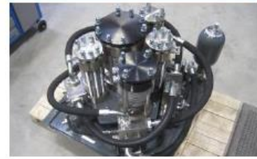
Compression (e.g. ionic compressor station)
