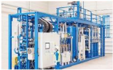
Steam reformer (e.g. steam biomethane reformer)
